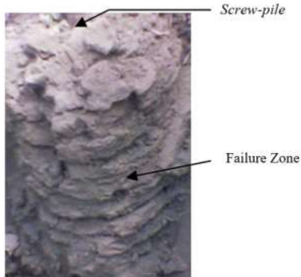
Figure 3. Observed failure mode of screw-pile anchors during the field tensile pull-out test, showing the development of the failure surface and associated deformation pattern
