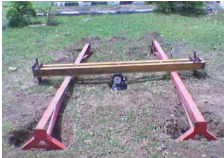
Figure 1. Tensile pull-out testing of screw-pile anchors
