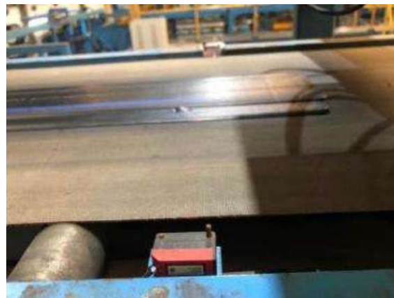
Figure 15. Photocell Sensor Design for Building a Tyre Machine
