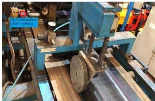
Figure 11. Photocell Sensor Placement Design
