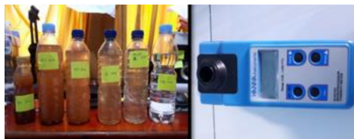
Figure 4. Turbidity Calibration with Hanna Instrument
